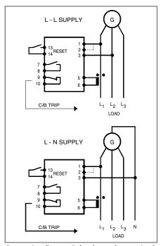
Connection diagram. Relay shown de-energized.
